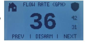
Flow needs to be above minimum flow rating shown on page 1 of this manual in order to arm.
