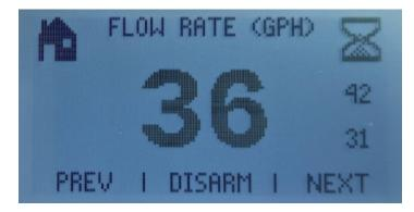
If the IS Lite is power cycled while armed or with an active alarm, a flashing hour glass icon will show in the top right corner of the display for the length of the Power On Delay Time.
