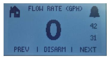
If flow goes outside of the flow window a flashing alarm bell icon will show in the top right corner of the screen.
